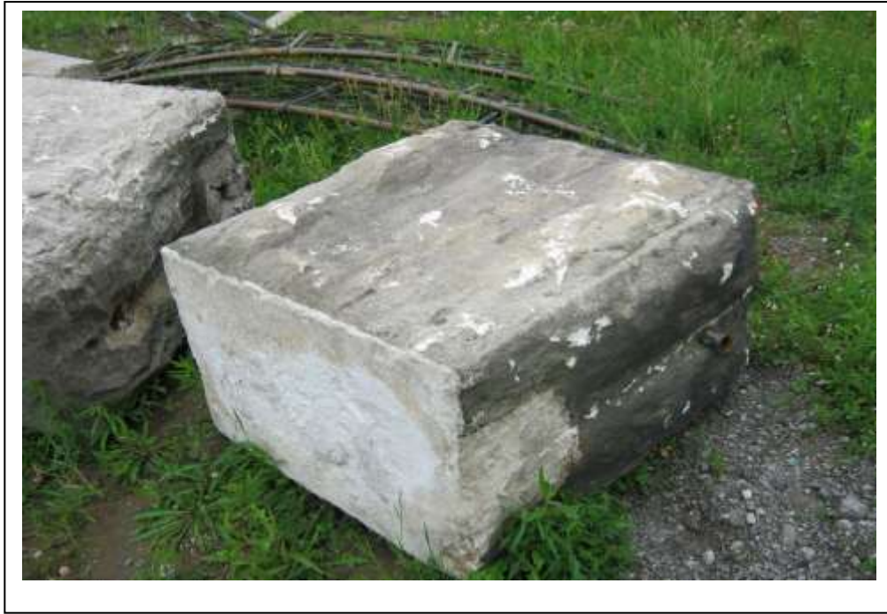
Fig.2: Potential salvaged stone #2 from the old bridge. (40" tall x 36" wide x 24" deep)
